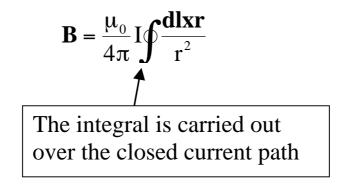
dl is an integration element of length along the current path
