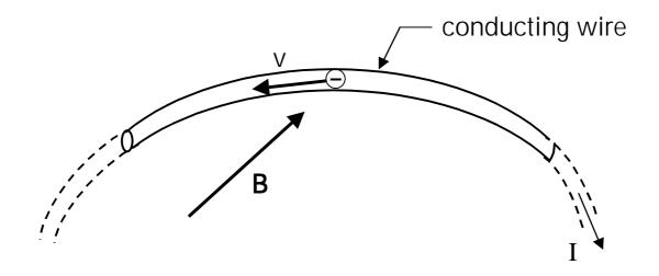
A conducting wire contains about n  $\sim 10^{28}$  -  $10^{29}$  conduction electrons per m<sup>3</sup> of metal. Each electron experiences a force
