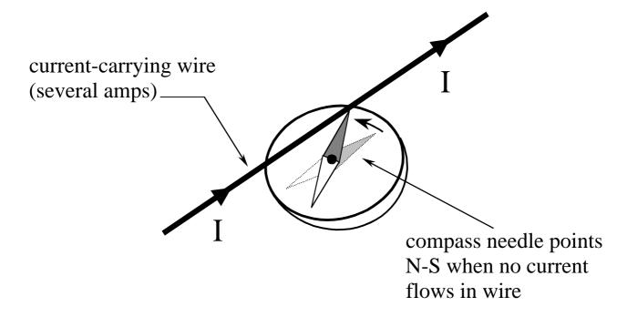
Lecture demonstration: Oersted's experiment (compass deflected by current carrying wire)
