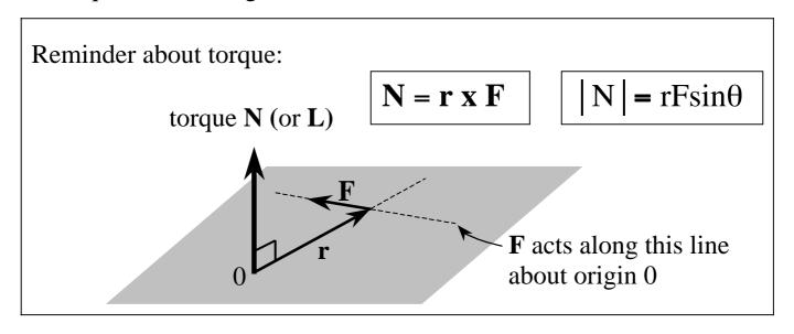
Take a rectangular current-carrying loop (it's easier than the circular loop we are interested in) and find the torque on it in a magnetic field B in the z-direction:
