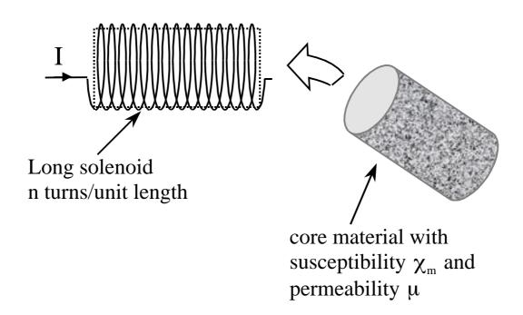
The magnetic induction  ${\bf B}$  inside the solenoid has contributions from free currents, I and equivalent bound current densities,  ${\bf K}_b$  and  ${\bf J}_b$  (arising from the magnetization of the core material).
